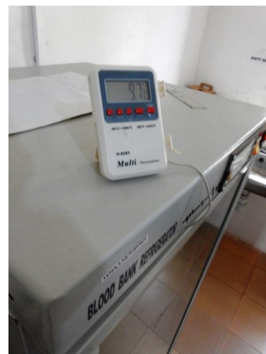
Bloodbank fridge with too high temeparature
